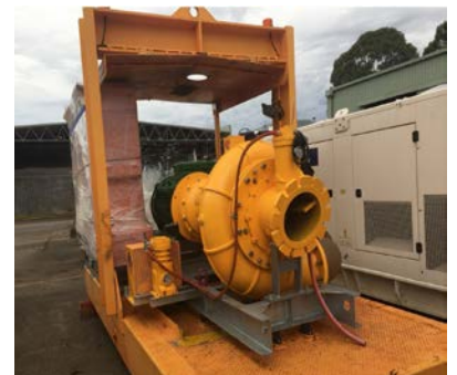
Sykes unit converted to electric power
