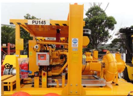
Original Sykes diesel powered unit
