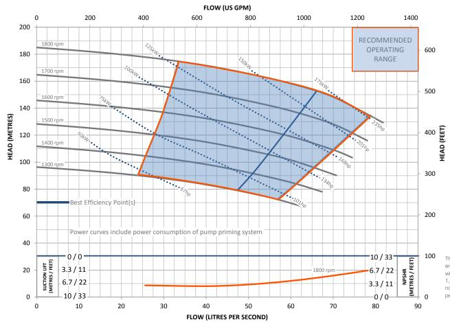
This pump and engine combination will produce up to 1,700 RPM of non-overload pump performance.
