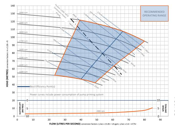
This pump and engine combination will produce up to 1,600 RPM of non-overload pump performance.
