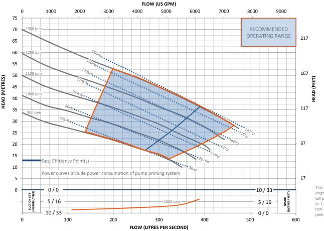
This pump and engine combination will produce up to 1,200 RPM of non-overload pump performance.
