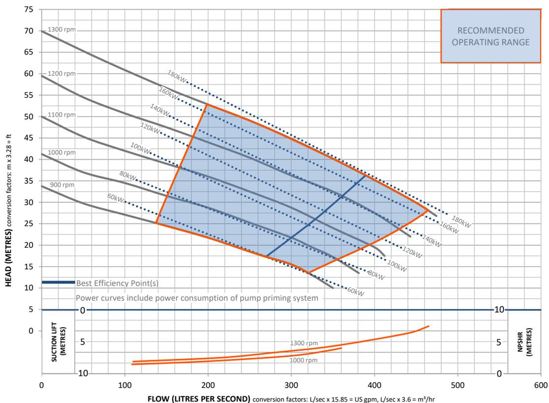
Max 1200 rpm with 1106D-E70TA engine
