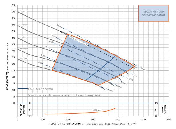
This pump and engine combination will produce up to 1,200 RPM of non-overload pump performance.
