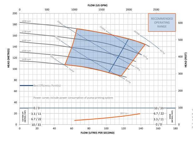
This pump and engine combination will produce up to 1,800 RPM of non-overload pump performance.
