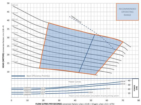
This pump and engine combination will produce up to 1,950 RPM of non-overload pump performance.
