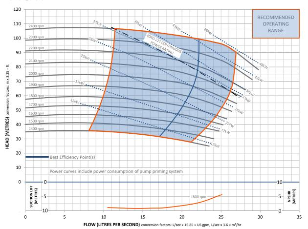
This pump and engine combination will produce up to 2,000 RPM of non-overload pump performance.
