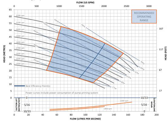
This pump and engine combination will produce up to 2,200 RPM of non-overload pump performance.
