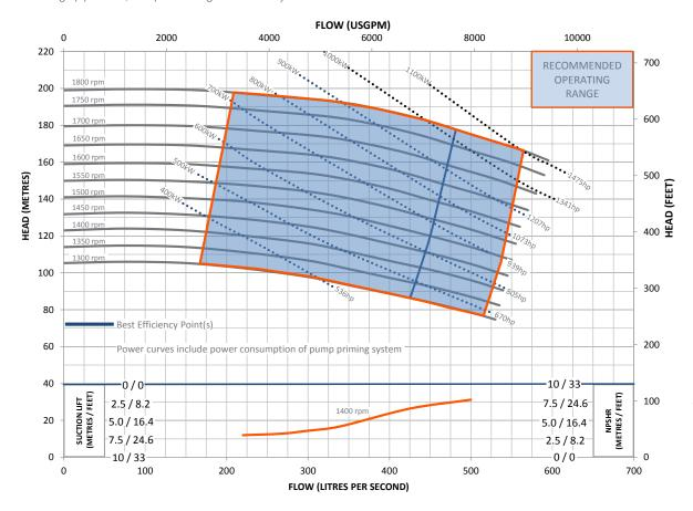
This pump and engine combination will produce up to 1,450 RPM of non-overload pump performance.
