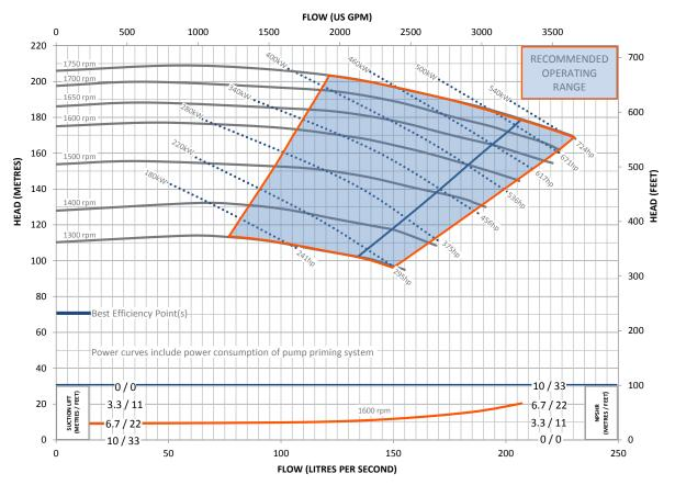
This pump and engine combination will produce up to 1,750 RPM of non-overload pump performance.
