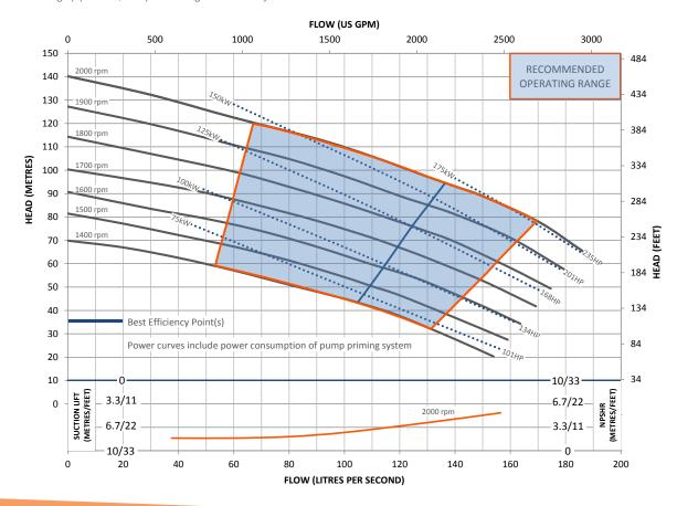
This pump and engine combination will produce up to 1,900 RPM of nonoverload pump performance.
