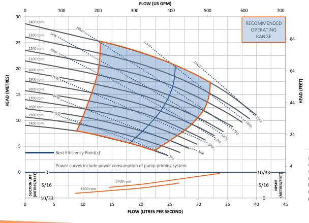
This pump and engine combination will produce up to 2,400 RPM of nonoverload pump performance.
