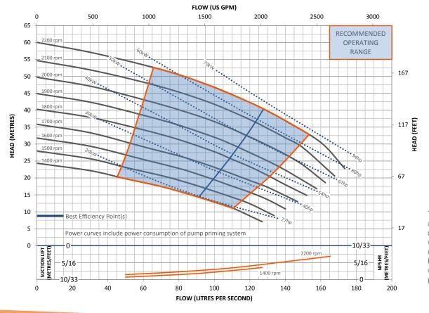
This pump and engine combination will produce up to 2,200 RPM of nonoverload pump performance.
