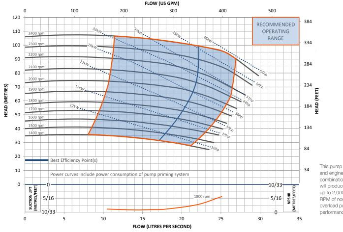
and engine combination will produce up to 2,000 RPM of nonoverload pump performance.
