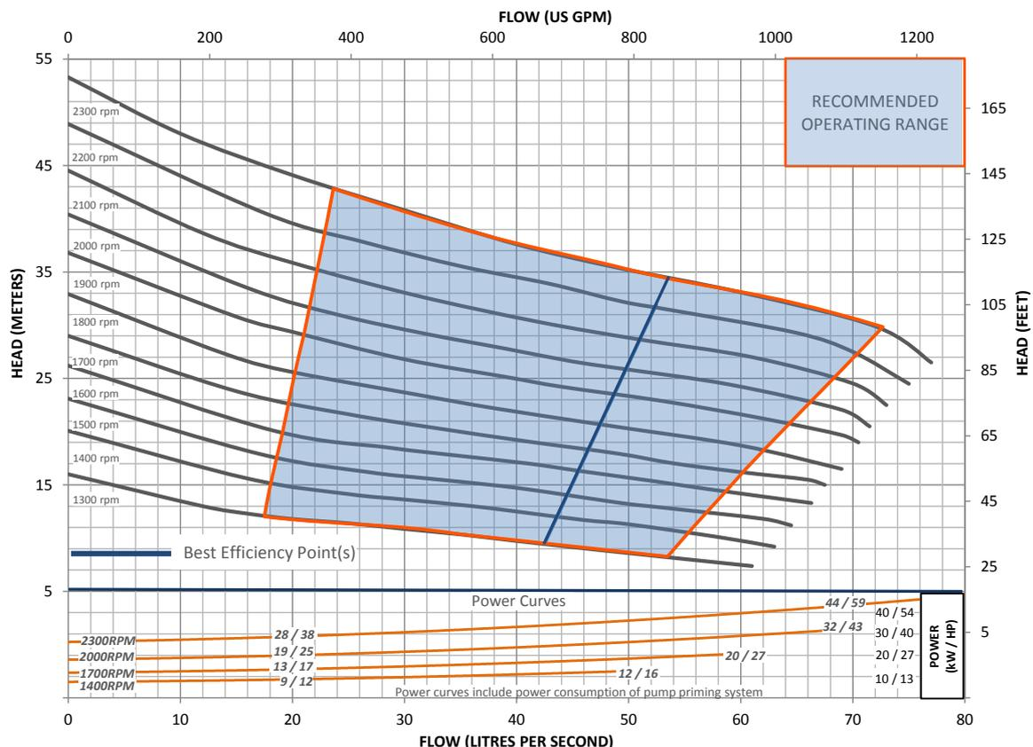
This pump and engine combination will produce up to 2,100 RPM of non-overload pump performance.
